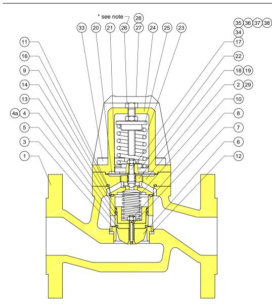
\*Adjust the nut on top of spring cap – not the adjusting screw head.
