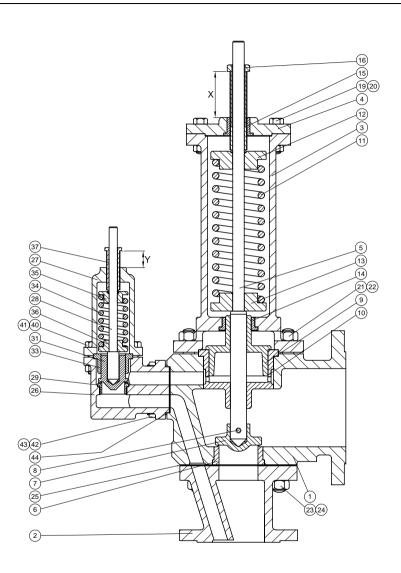
Before any work is carried out on the valve carefully measure dimensions 'X' and 'Y' and ensure that the valve is totally isolated from any pressure in the pipeline. Do not attempt to strip valve without first relaxing the compression on the springs.
