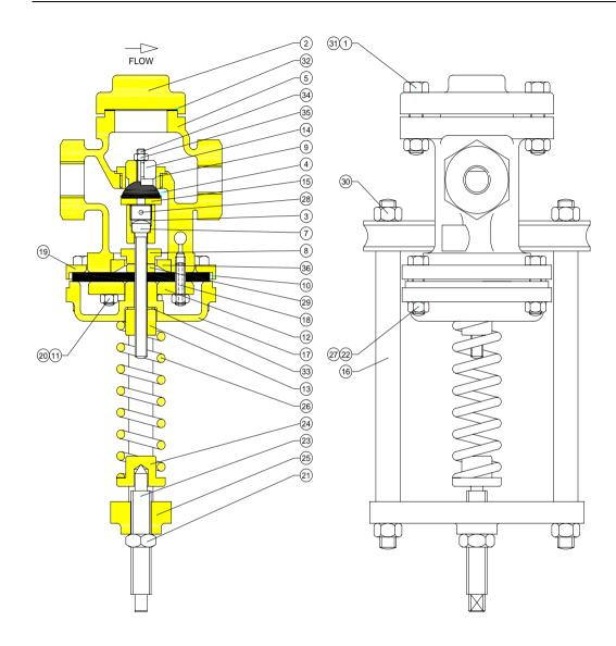
Before any work is carried out on the valve ensure that the valve is totally isolated from any pressure in the pipeline. Do not attempt to strip valve without first relaxing the compression on the spring.
