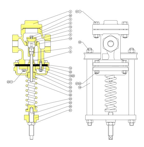
Before any work is carried out on the valve ensure that the valve is totally isolated from any pressure in the pipeline. Do not attempt to strip valve without first relaxing the compression on the spring.
